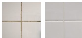
The product was sprayed onto ceramic tiles and grout stained with mold. The product was left to sit for 5 minutes and then the final image was taken (no scrubbing)
